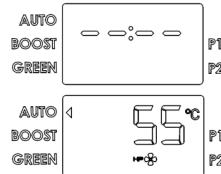
**Turning the appliance off:** simply press the ON/OFF button to turn the water heater off, only "OFF" appears on the display. The protection against corrosion is still ensured, while the product will automatically ensure that the temperature of the water in the tank does not fall below 5°C.
