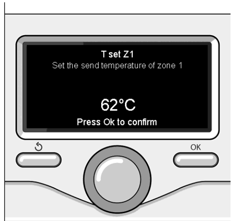
Change heating hot water temperature
