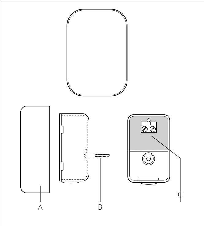
Position the outdoor sensor on the north-facing wall of the building, at least 2.5 m from the ground and away from direct sunlight.
