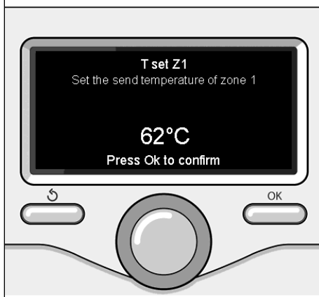
Change heating hot water temperature
